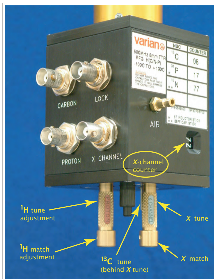
Figure 7.2 The Varian HCX triple-resonance probe: external tuning mechanisms
